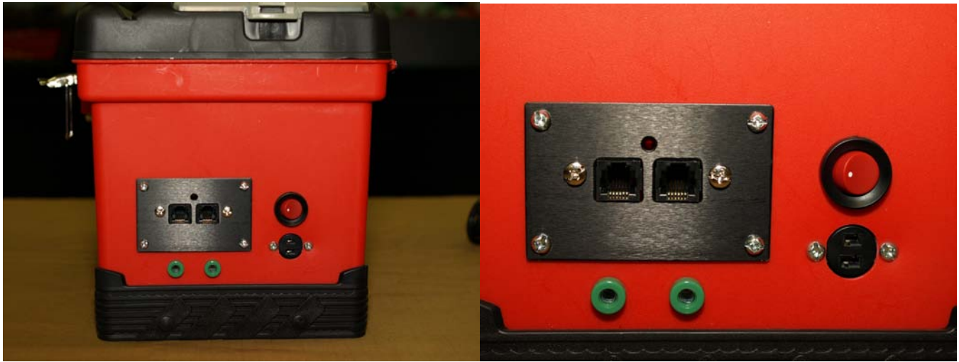
Figure 9 – Completed Output End Connections
