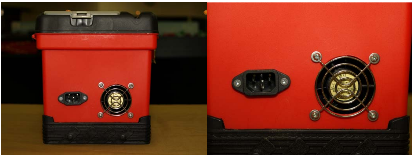
Figure 10 – Completed Input End Connections
