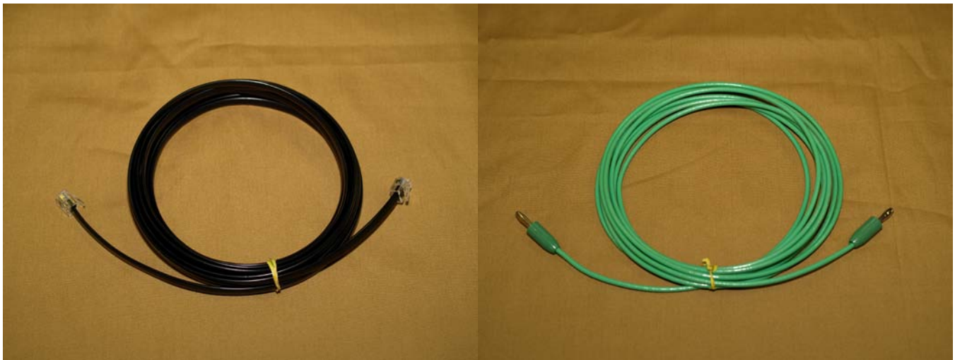
Figure 12 – Loconet and Ground Cables
